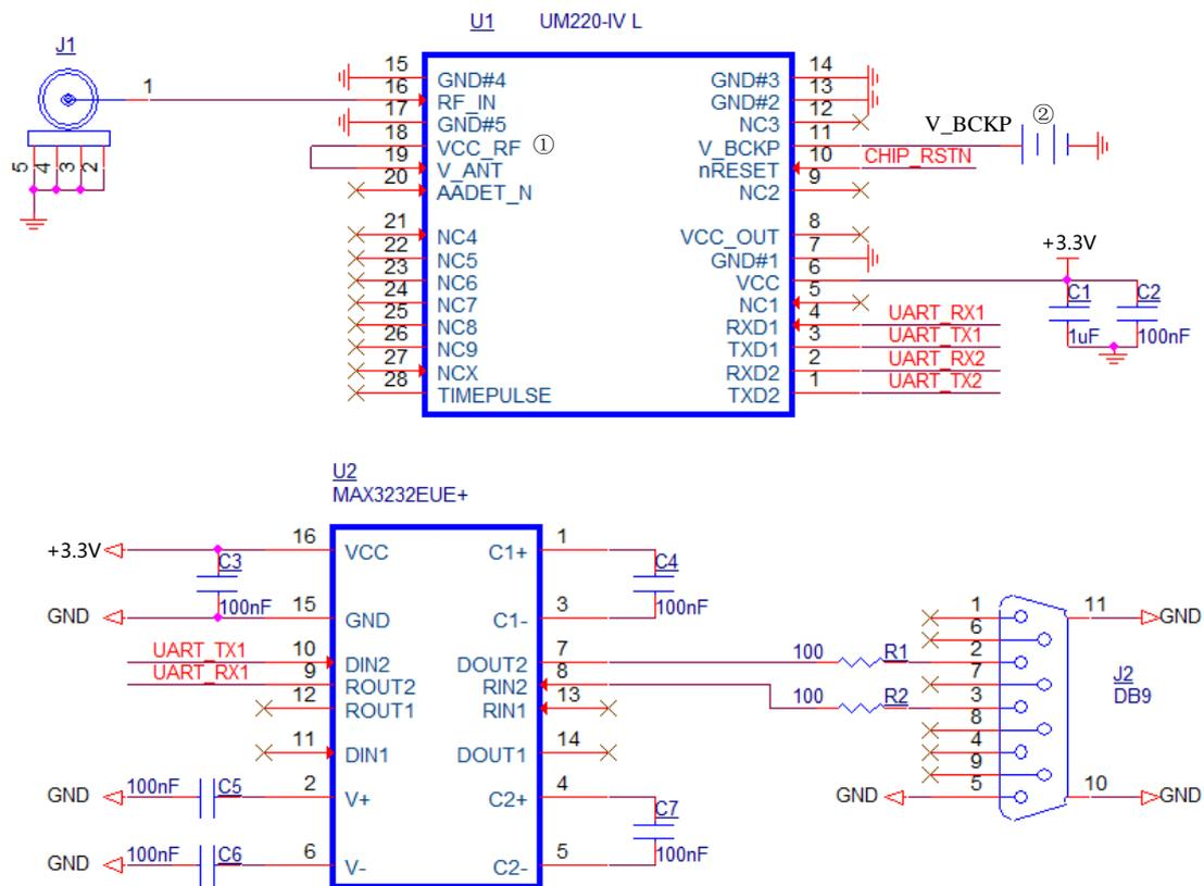
Figure 1-1 Minimum System Reference Circuit
