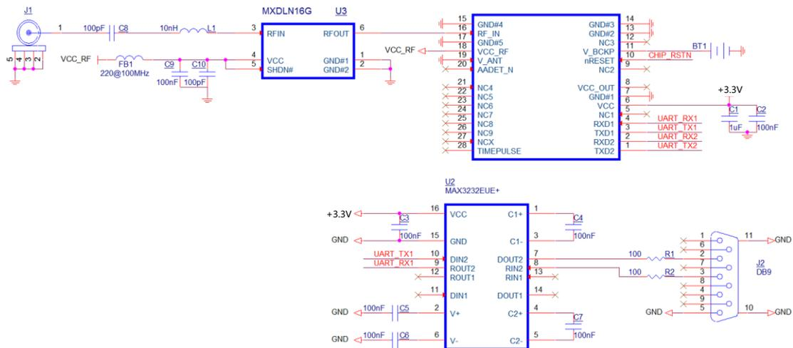
Figure 2-1 Reference Circuit Using a Passive Antenna
